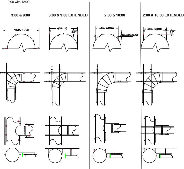
Note: The previous drawings illustrate possible double cable suspension systems. Some installations may require cable support brackets. Since every installation is different, support brackets are not supplied. Triple suspension systems used on larger diameters systems would be a combination of both single and double suspension guidelines.
