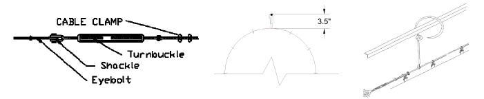
When fabric fittings are incorporated in your installation, align cables with the centerline of the system. All cables should be installed at the same elevation.
